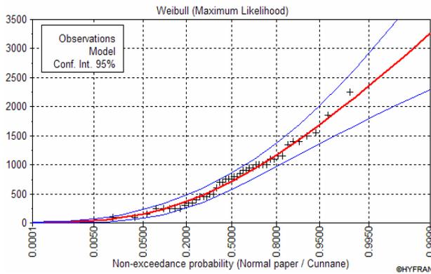
**Figure 4. Theoretical curve for estimation of irrigation norms for first year spruce seedlings, with different probability years**
