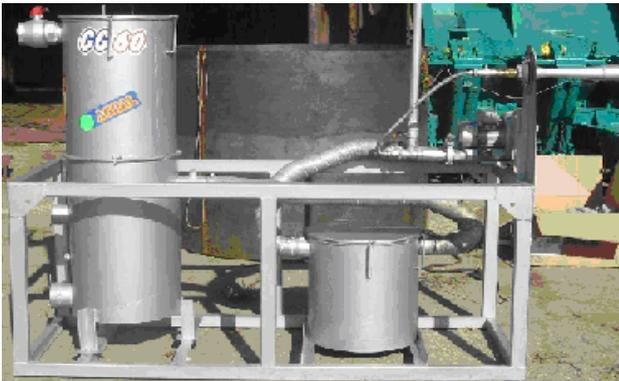
**Figure 1 – The heating plant GG-60 using generator gas**
